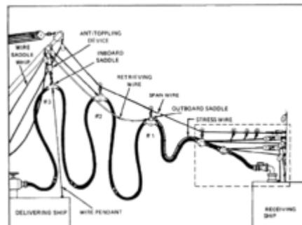
Span-wire fueling rig as used since 1945
