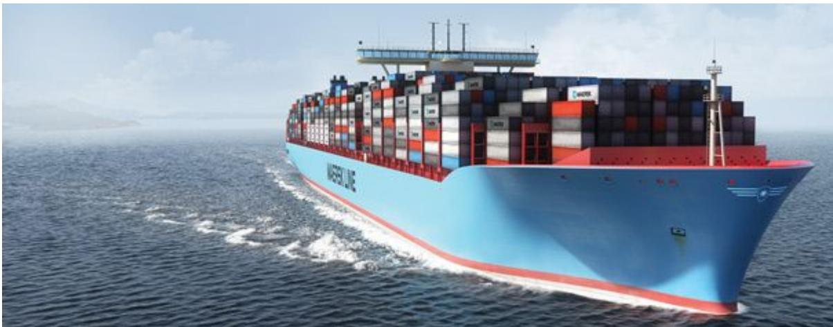
The Triple E's bridge has been brought forward so containers can be stacked higher with no loss of visibility
